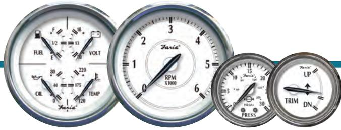
Perimeter lighted white dial with classic black and grey graphics, hand-polished stainless steel bezel, domed fog resistant lens and two piece pointer. Instruments illuminate red for improved low light visibility and connection type is studded.
